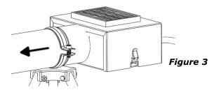
d. Tighten barrel clamp bolts with the provided 6mm wrench.
